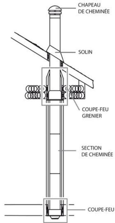
Figure 46: Installation standard
