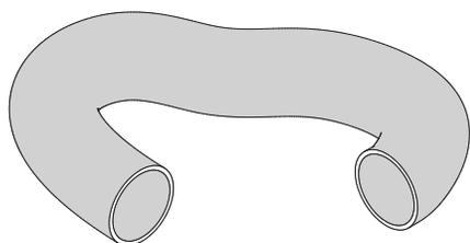
Tuyau isolé flexible de type HVAC
